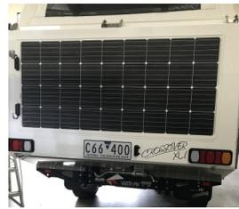
Rear mounted 215 Watt 12VDC Mono Flexible Solar Panel with Anderson plug input for additional solar arrays
