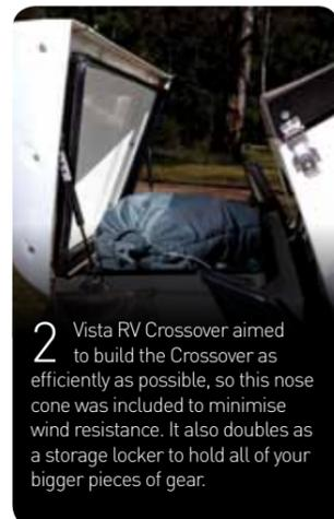
**2** Vista RV Crossover aimed to build the Crossover as efficiently as possible, so this nose cone was included to minimise wind resistance. It also doubles as a storage locker to hold all of your bigger pieces of gear.
