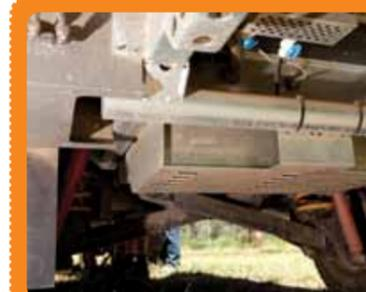
**10** The underside of the Vista RV Crossover is where the unit really shines. The heavy-duty chassis and on-board water tank, which is permanently plumbed in, and independent suspension set a high benchmark that the body of the Crossover follows closely.
