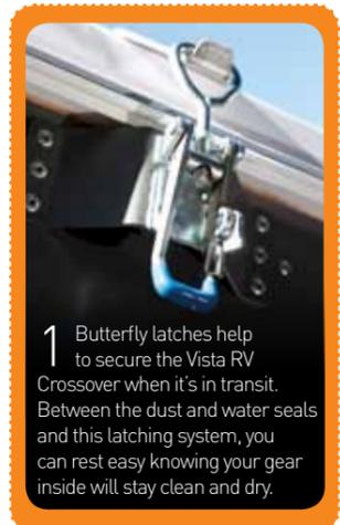
**1** Butterfly latches help to secure the Vista RV Crossover when it's in transit. Between the dust and water seals and this latching system, you can rest easy knowing your gear inside will stay clean and dry.
