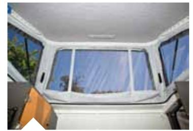
The top of the TVK expands to reveal flyscreen mesh that allows for effective airflow and ventilation. This is the perfect way to keep cool on hot summer nights, and provide some additional headroom for taller campers
