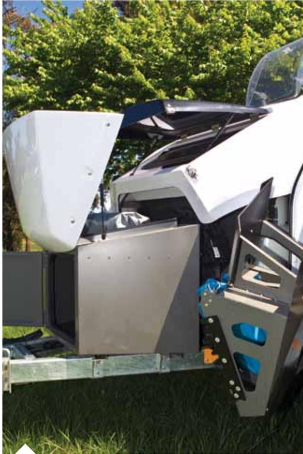
The front end of the TVK is compact, yet houses plenty of gear in a robust way. A front boot has dual access compartments that give way to the composite constructed body of the camper. From here, an additional storage space opens up to house anything that would be out of place if stored internally, such as wet clothes or tools. A hatch is located at the top of the TVK to allow for plenty of ventilation, which is great for those warm, remote locations
