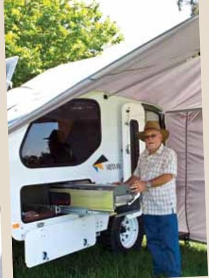
An awning extends easily from the body of the trailer on telescopic poles. Awnings provide an additional living space, which is a great asset if you're housing a large family in a small camper for an extended period of time. Keep in mind that they can be cumbersome to set up if they're after market, so it's best to get one that fits well from the factory wherever possible
