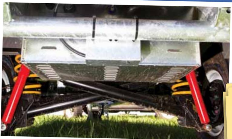
Once you climb underneath the TVK, it really comes to life. The Crossover MS suspension series has been designed specifically for Vista RV's campers, and is used across the board with all of the campers it offers. It gives plenty of flex, with up to 330mm of travel at each wheel – great for the tougher tracks
